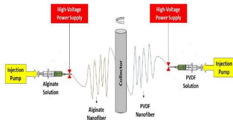
The schematic figure of the electrospinning process. The polymer solutions are poured in the syringes; in this method high-voltage electricity is used to draw charged threads of polymer solutions to fiber diameters.
