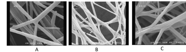
Figure 1: **A:** PVDF based scaffold. The average fiber diameter in this scaffold was 95.22 nm. **B:** Crosslinked Alginate/PVDF scaffold. The average Alginate fiber diameter in this scaffold was 59.93 nm and PVDF fiber diameter was 104.55 nm. **C:** Non-crosslinked Alginate/PVDF scaffold. The average Alginate fiber diameter in this scaffold was 51.4 nm and PVDF fiber diameter was 131.81 nm
