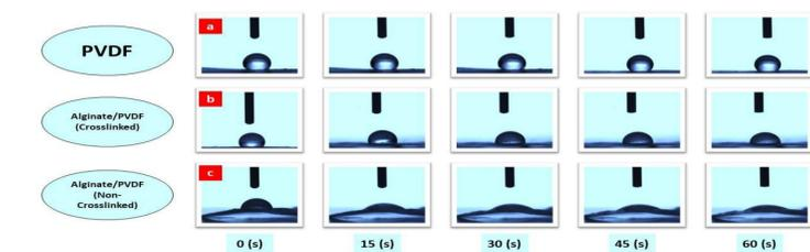
a: the PVDF based scaffold showed a hydrophobic characteristic and the shape of the water drop did not change during the test time. b: The crosslinked Alginate/PVDF scaffold showed better hydrophilicity and c: the non-crosslinked Alginate/PVDF scaffold had the highest hydrophilicity and the water drop had completely lost its drop shape.
