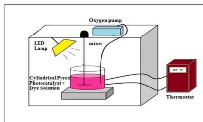
Fig. 2. Schematic of the photocatalytic experimental.
