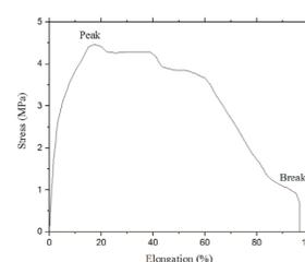
Figure 3. Stress-elongation of polyvinyl alcohol / graphene-copper-curcumin
