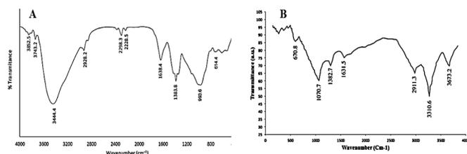
Figure 1. FTIR spectra of A) GO/Cu/Cur , B) PVA/GO/Cu/Cur
