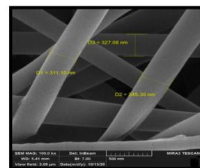
Figure 2. Scanning electron microscope (SEM) image of PVA/GO-Cu-Cur nanofibers
