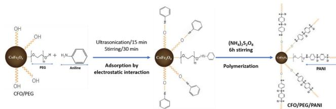
Figure 1: Schematic illustration of the fabrication of CFO/PEG/PANI.
