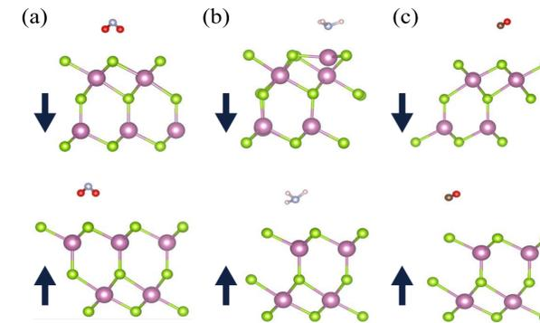
Figure 2: Most stable structure for the adsorption of various gas molecules on different surfaces of In<sub>2</sub>Se<sub>3</sub>: (a) NO<sub>2</sub>, (b) NH<sub>3</sub>, and (c) CO adsorption.
