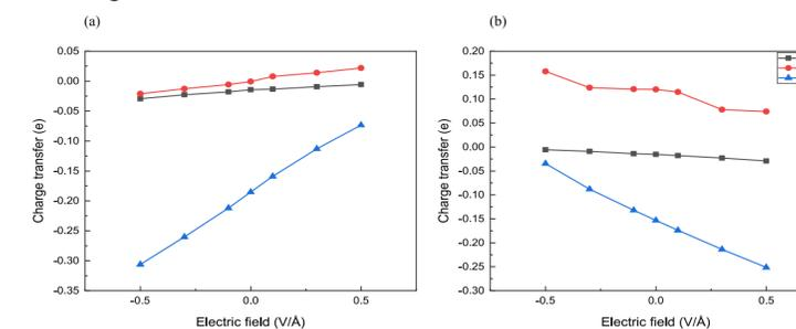
Figure 4: Electric field effects on charge transfer of CO, NH<sub>3</sub>, and NO<sub>2</sub> molecules adsorbed on (a) up and (b) down sides of In<sub>2</sub>Se<sub>3</sub> monolayer.
