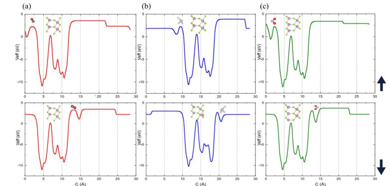
Figure 5: Electrostatic surface potential (ESP) for (a) CO, (b) NH<sub>3</sub>, and (c) NO<sub>2</sub> gas molecule adsorption on up and down sides of In<sub>2</sub>Se<sub>3</sub> monolayer.
