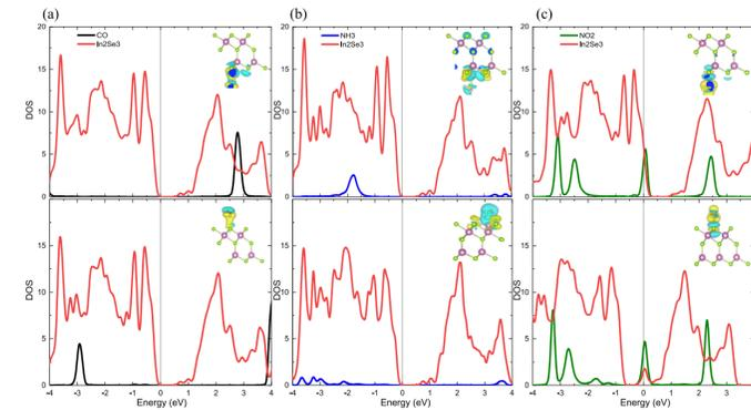
Figure 3: The PDOS of (a) CO, (b) NH<sub>3</sub>, and (c) NO<sub>2</sub> molecules adsorbed on In<sub>2</sub>Se<sub>3</sub> monolayer for up and down sides.
