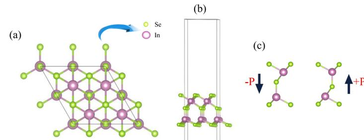
Figure 1: a schematic illustration of (a) top, and (b) side view of In<sub>2</sub>Se<sub>3</sub> monolayer used for our calculations. (c) Two stable structures of In<sub>2</sub>Se<sub>3</sub> which can be switch to each other by laterally moving the central Se atom and reorientation of top In atoms. Both surfaces have spontaneous electric polarization with opposite directions. Up and down arrows refer to positive and negative polarizations, respectively.
